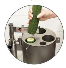
Best for: To be able to easily cut long and narrow products vertically, and round products in a specific direction, the cutting cylinder is used. Good support for products such as cucumbers and leeks. It is also easy to "bunch" herbs together in the tube. This feeder has 4 tubes:
