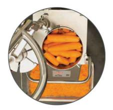
Best for: The stacking cylinder can prepare all types of products, both large and small. The Ergo-loop design provides a lever effect that also reduces the need for manual force when preparing large and hard products, such as root vegetables, cabbage and cheese.
